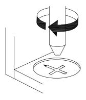
**EN**\_Turn cam lock clockwise to tighten.
